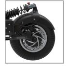
If that happens, clean the inner surface of the disc by turning the wheels with a clean, dry cloth and straighten any bent discs.
